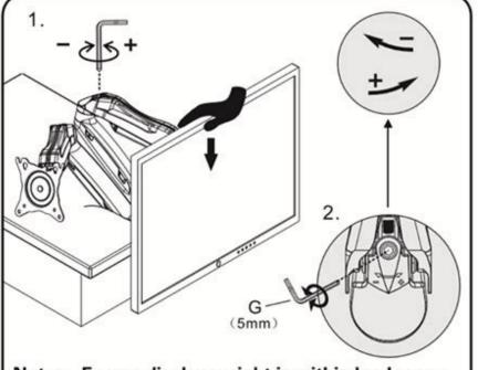
Notes: Ensure display weight is within load range. 1.If display can be hovered at any height after display installed.
